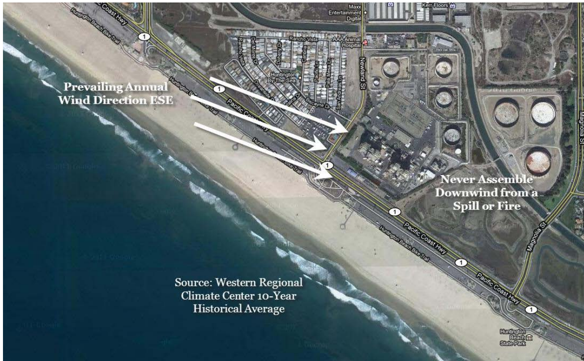
Plant Prevailing Wind Information (ALWAYS ASSEMBLE UPWIND)
